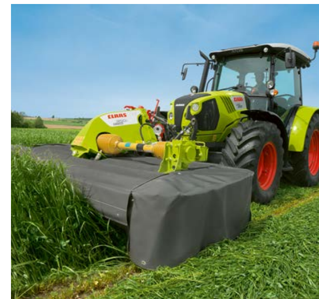
▲ Compact hitch at the front linkage gives the DISCO PROFIL generous ground clearance at the headland
