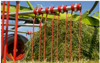
Silage tines for gentle forage handling
