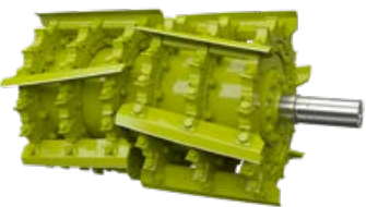
▲ One third set of knives (with V-36 only) for very long lengths of cut with symmetrical crop discharge.
