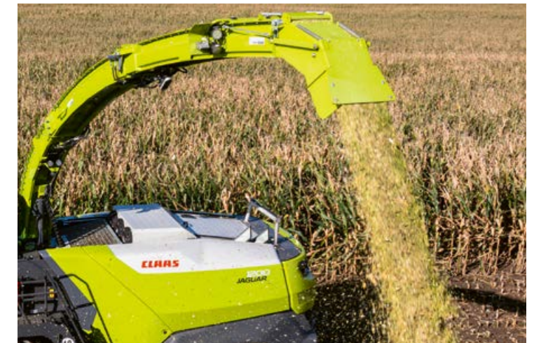
▲ With its large cross-section, the discharge spout is designed to deliver high throughput reliably. Page 28
