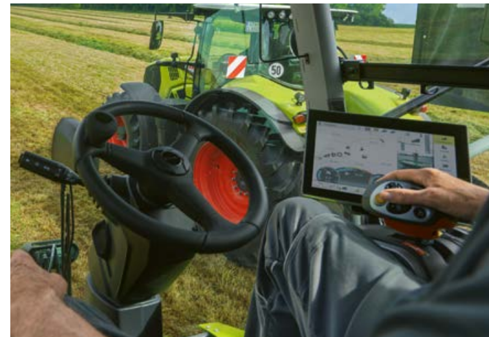
▲ CEMOS maintains the engine speed set by the operator and adjusts the engine output and ground speed in accordance with the volume harvested. CEMOS AUTO CROP FLOW provides overload protection. Page 42
