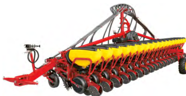
Equipped with transport wheels and a drawbar, Tempo R 12-18 can be easily transported between fields.
