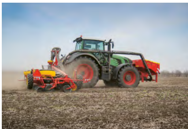
The front mounted fertiliser hopper FH 2200 enables high precision combi-drilling.
