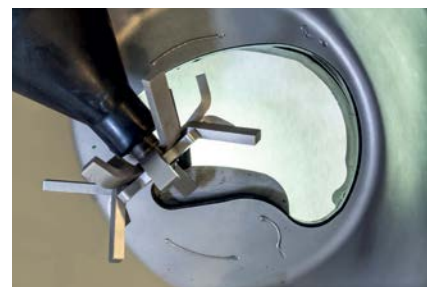
Stage 3: hopper aperture wide open
