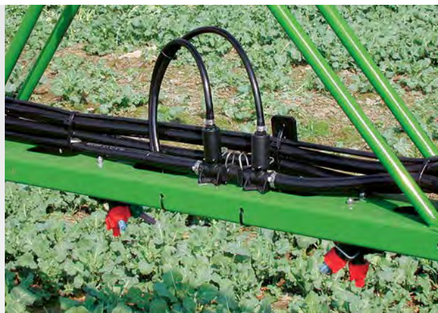
DUS pressure recirculation system
