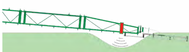
DistanceControl when equipped with two sensors: the boom can dip into the crop, for example, where there is lodged corn
