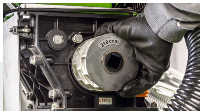
Easy exchange of the metering rollers
