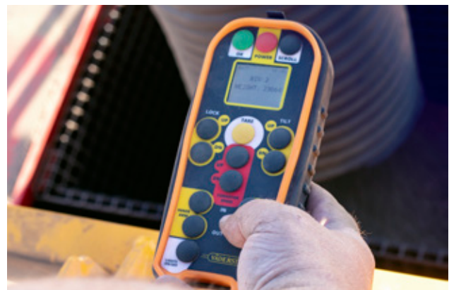
New fill system remote for 800 & 980 Air Carts allows for more functionality including belt speed controls while displaying real-time load cell values for each bin.
