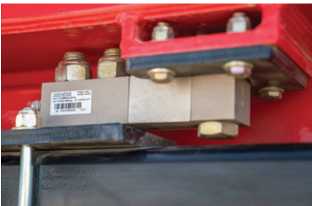
The modular tank design of Seed Hawk Air Carts features individual compartment load cells.
