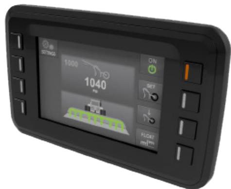
New Toolbar Control System (TCS) for pairing with off-brand carts comes with stand alone 5" touch screen.
