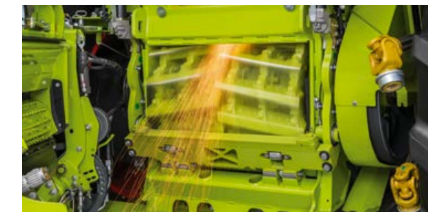
Sharpening and adjusting the shear bar takes hardly any time at all.
