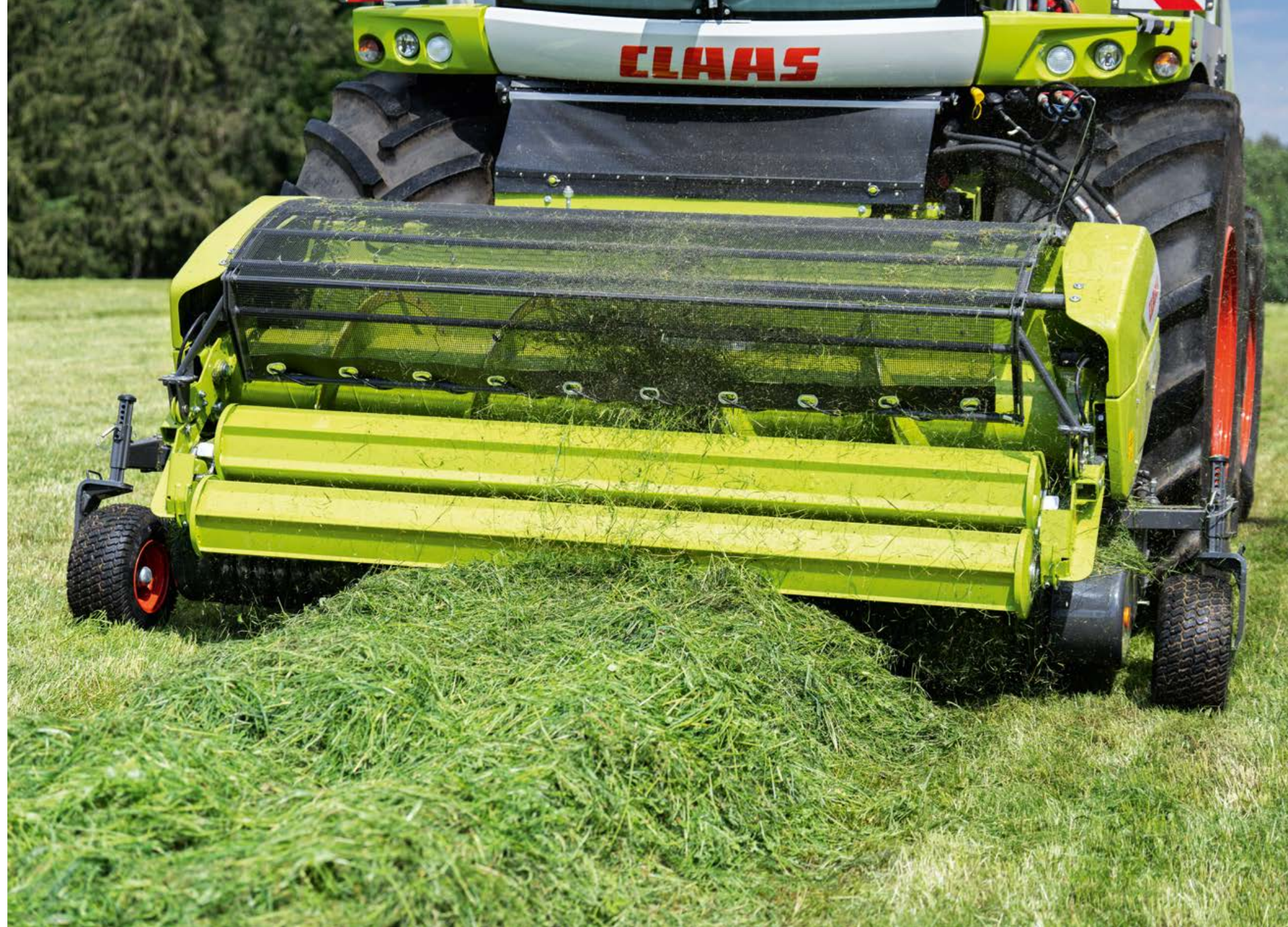
Intake auger with four paddles.
