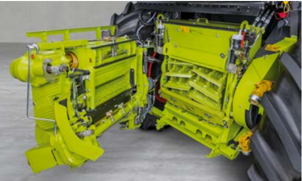
Easily accessible chopping cylinder for quick and easy maintenance.
