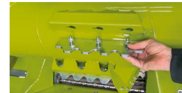
Intake auger with four paddles.
