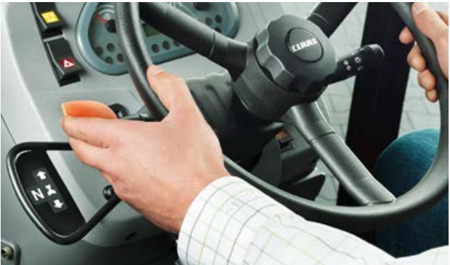
1 REVERSHIFT lever for rapid and comfortable turning manoeuvres, particularly at headlands or when stacking boxes.
