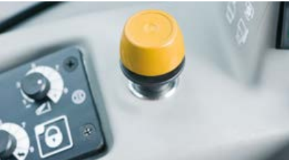
Electrohydraulic PTO engagement/disengagement
