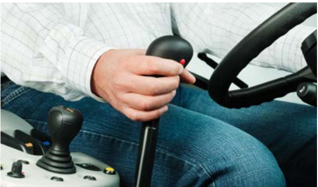
1 REVERSHIFT lever for rapid and comfortable turning manoeuvres, particularly at headlands or when stacking boxes.
