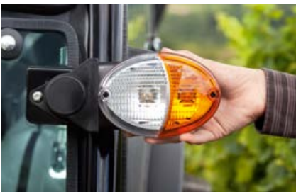
Folding side-marker lights on the NEXOS VE prevent damage to crops
