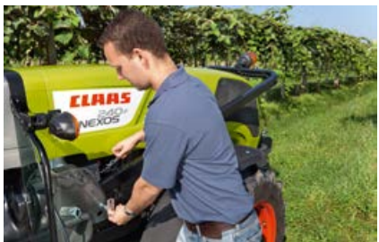
The roll bar can be folded down in no time with no need for tools
