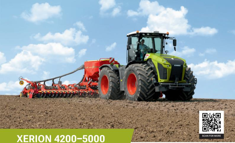
Uniquely designed for maximum slip control, tractive performance, and dynamism. A Mercedes-Benz engine efficiently delivers up to 530hp from a CMATIC continuously variable transmission, with four equal-sized wheels or dual tyres that convert engine power into tractive power. Intelligent systems combined with intuitive operation via the CEBIS touchscreen display, well-appointed suspended cab with excellent visibility, and long service intervals, XERION tractors are unbeatable in the field.
