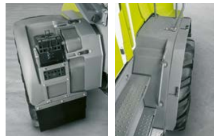
All mudguards on all TORION models in the medium series are optionally available adjustable to improve visibility of the wheels, especially when working along silage clamp walls.
