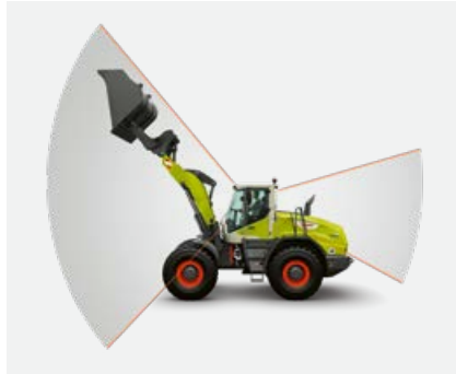
The slim pillars grant an unobstructed view of the implement carrier.
