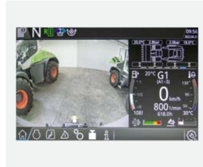
The rear camera is activated automatically as soon as you shift into reverse.
