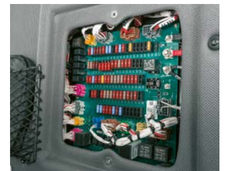
The on-board electronics is bundled for easy access.
