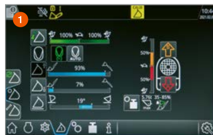
The lifting and lowering height limits store the ideal level close to the ground and the dumping height.
