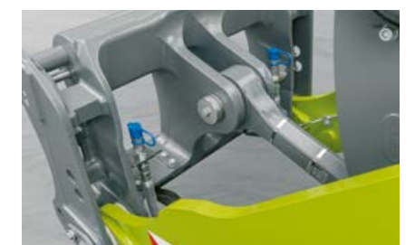
The machine is prepared for two more hydraulic connections.
