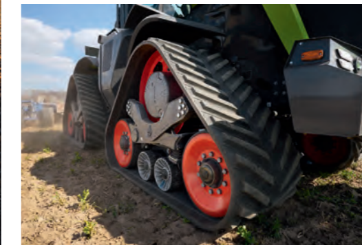
◀ Two belt widths (914 mm or 762 mm) guarantee maximum ground protection. With the narrower track belts, the overall width of the XERION is less than 3 m.
