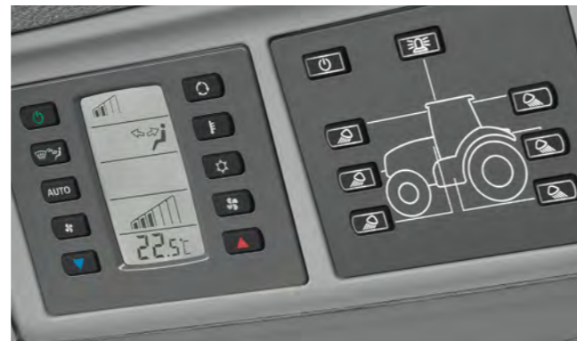
As well as the manually controlled air-conditioning system, a fully automated version is available which provides a pleasant flow of air through the cab.
