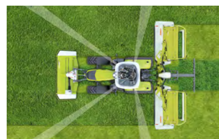
The cleverly positioned rear cab pillars and convex rear window give the driver an excellent view of the implement and hitch area.
