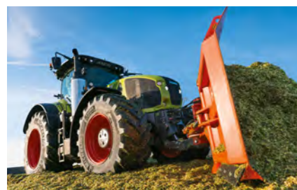
When a front linkage is installed, up to two double-acting spool valves and one free-flow return line are available at the front. Ideal for a front-mounted seed hopper or dozer blade.
