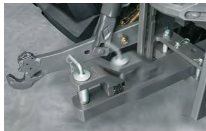
The drawbar versions offer several positions. The extended position increases manoeuvrability.
