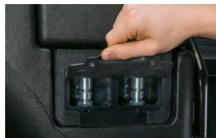
External battery terminals are within easy reach by the left-hand cab access ladder.
