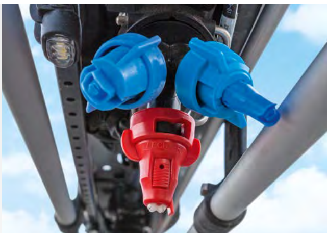
✔ AmaSwitch electric single nozzle control
