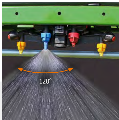
AmaSelect electric single nozzle control with a 4-fold nozzle body and 50 cm or 25 cm nozzle spacing
