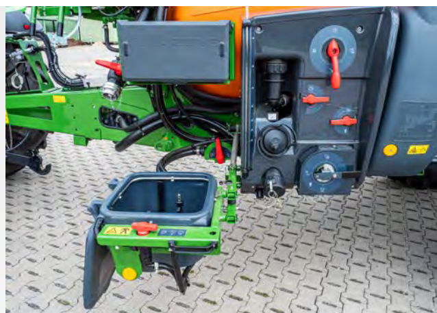
SmartCenter on the left hand side of the machine with the induction bowl folded out
