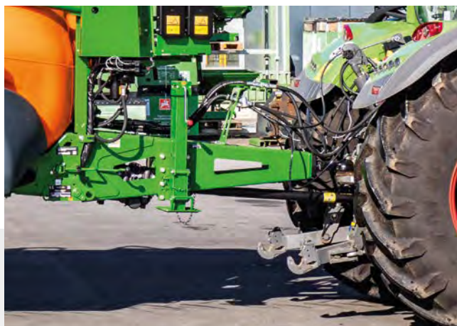
Top mounted drawbar with ball coupling and mechanical parking jack
