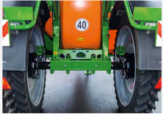
Adjustable axle with stepless track width adjustment from 1.50 m to 2.25 m
